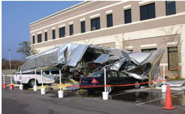
18,000 lb HVAC unit secured to curb with 16 straps, one screw per strap. Wind speed 85-90 mph
