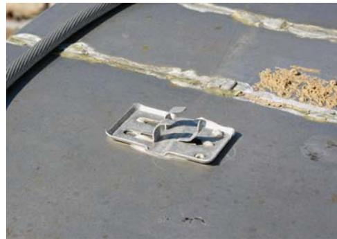
Conductor separated from clip after high wind
